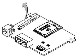
**IMPORTANT NOTICE:** Be sure the yellow ID label (9-digit ID number XXXXXXXXX) located to the right of the RS-484 connector on front side of indoor transceiver enclosure and the ID number on the ScreenLogic Interface outdoor wireless transceiver are the same. See page 1 for label location.
